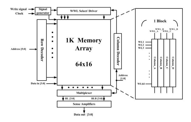
Fig. 3 . Architecture of proposed SRAM
