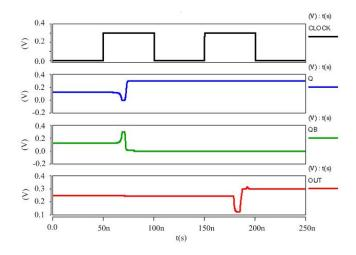
Fig. 4. Simulation Result in a write/read Operation Cycle (write "1" & read "1")
