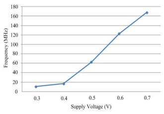
Fig. 5. Maximum operating frequency versus supply voltage
