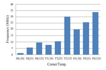
Fig. 6. Max operating frequency versus corner with different temperature
